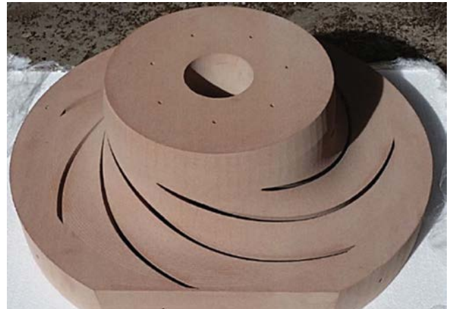
Figure 9: 3D sand printed impeller core. Photo courtesy of Saint Remy Industrie.
