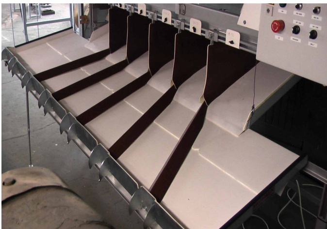
Exit on inclined plane
