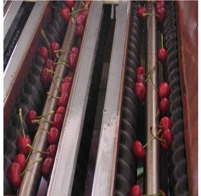
Main of the cherries take the same position on the screws
