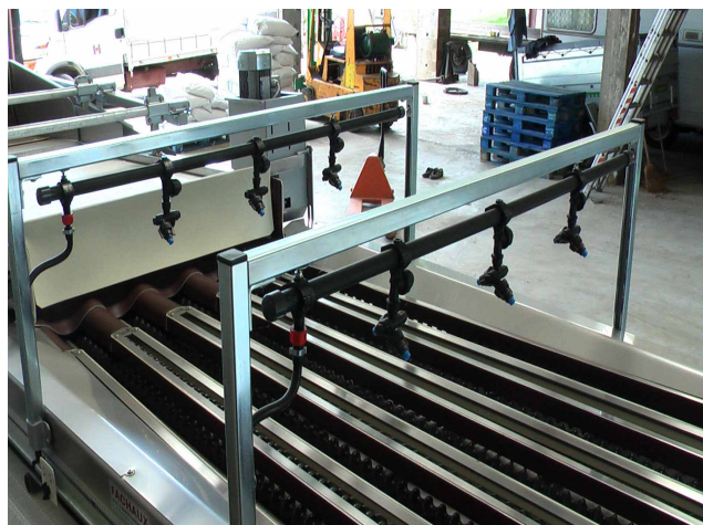
Water sprays over the sizer
